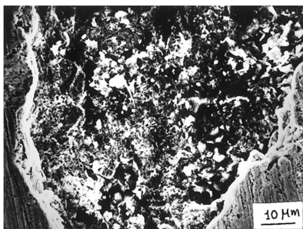
Fig. 4. SEM micrograph of alpha brass after immersion in 0.58 M NaCl + 2.5 \times 10^{-4} M (8 ppm) sulfide for five days.
